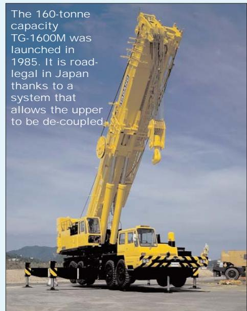
The 160-tonne capacity TG-1600M was launched in 1985. It is road-legal in Japan thanks to a system that allows the upper to be de-coupled
