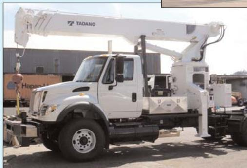
The new TM-20110 boom truck (above) has a maximum tip height of 120 feet. Like the established TM-1882 (left), it has the longest boom in its class.
