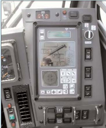
Tadano's Automatic Moment Limiter brings the boom slowly to a stop as it reaches working area limits, and so prevents loadsway
