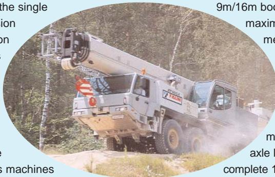
A key factor in its success was its pioneering 'Taxi' concept, coupled with the inclusion of a second engine for crane operations, making it the smallest twin-engine crane on the market.
