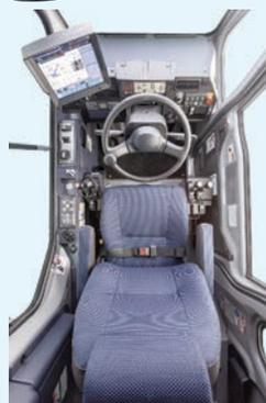
In terms of technology, introduction of the new generation Tadano automatic moment limiter AML-E replaces the current 5.7" black and white screen with a vibrant 10.4" color touchscreen for ease of use and better working condition visibility.
