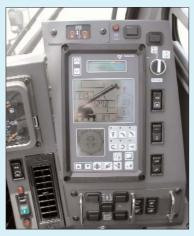
reached, it brings the boom to a gentle halt by slowing the boom elevation and telescoping cylinders. The rate of deceleration in each cylinder, and the point at which it begins, have been optimised to maximise safety and minimise disruption to crane productivity.
