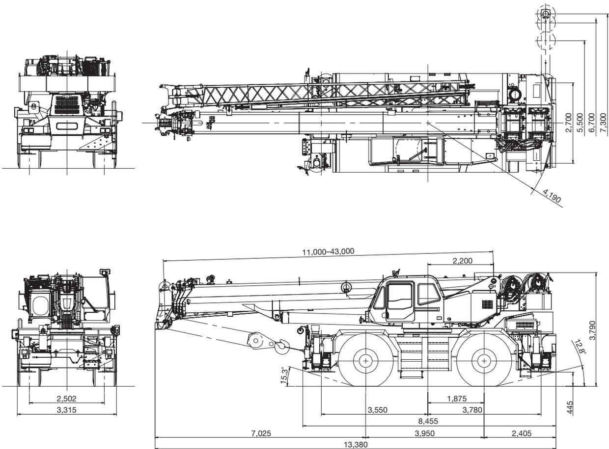
Note : Dimension is with boom angle at -1.6 degree.
