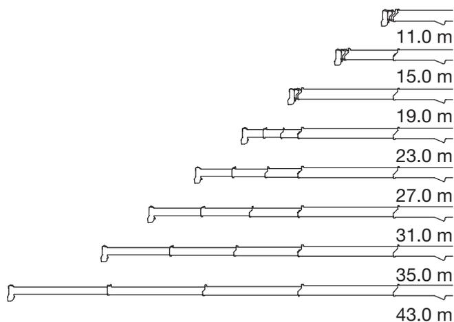
The above lifting height and boom angle are based on a straight (unloaded) boom and machine standing level on firm supporting surface. Allowance should be made for boom deflection obtained under loaded conditions. The above working range is shown on condition with outriggers fully (7.3 m) extended.
