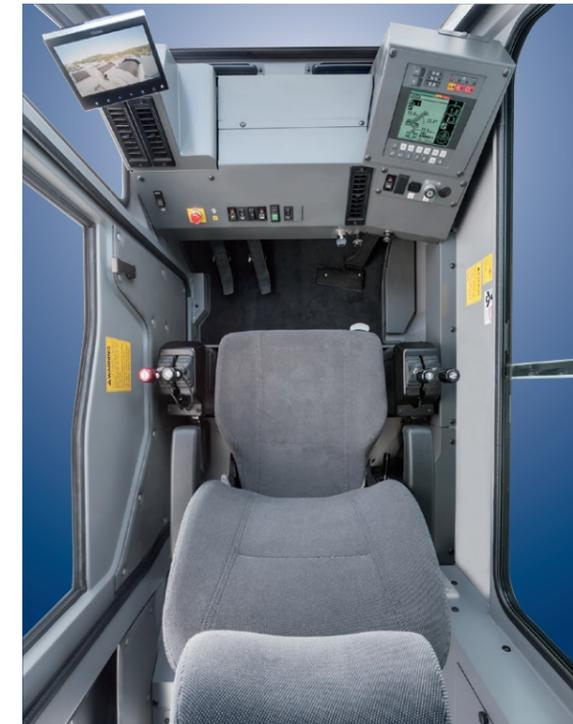
The crane operating levers are of finger control type and surely and steadily respond to the operator.
