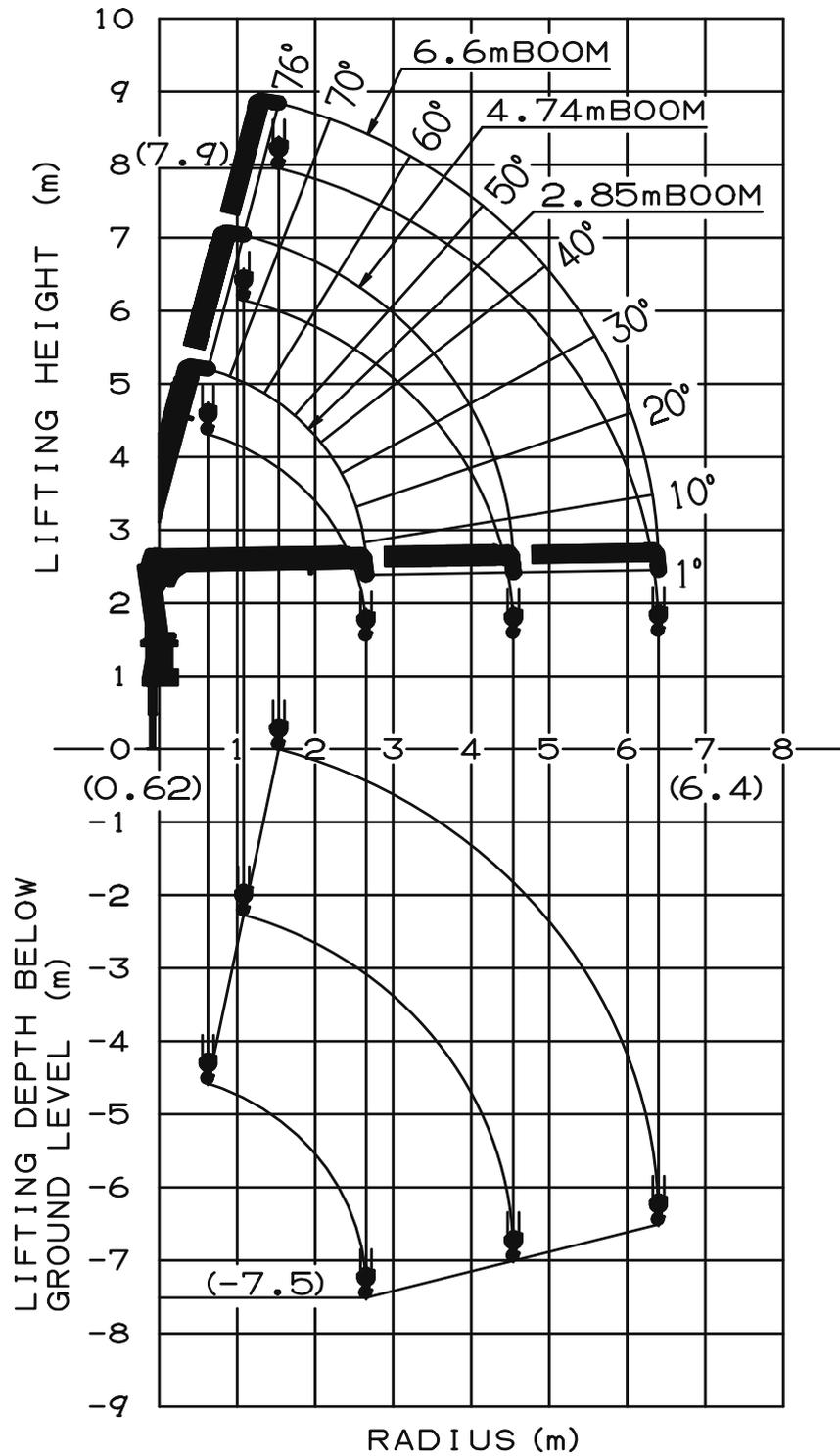
NOTE : The above lifting heights and boom angles are based on a straight (unladen) boom, and allowance should be made for boom deflection obtained under laden conditions.
