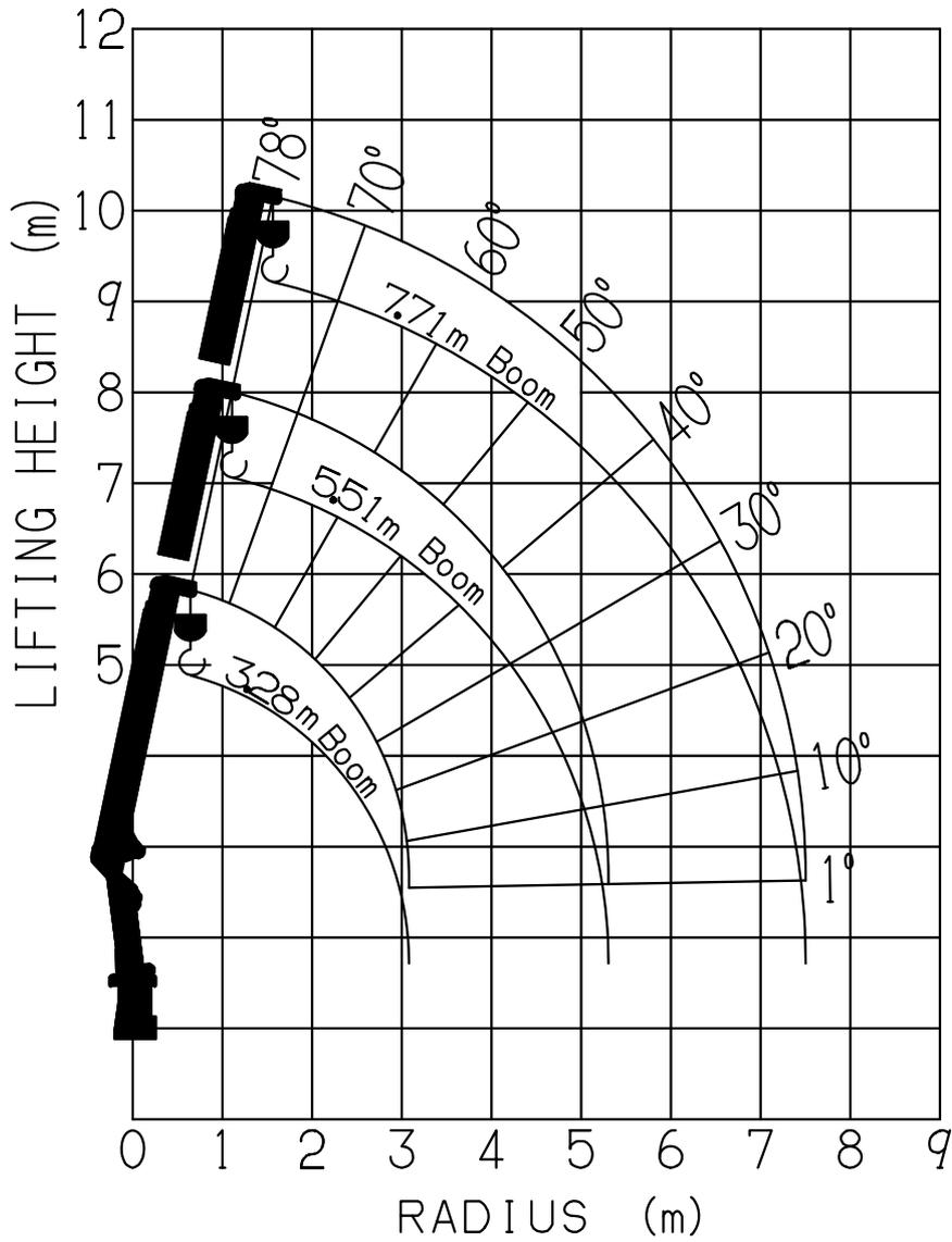
NOTE : The above lifting heights and boom angles are based on a straight (unladen) boom, and allowance should be made for boom deflection obtained under laden conditions.
