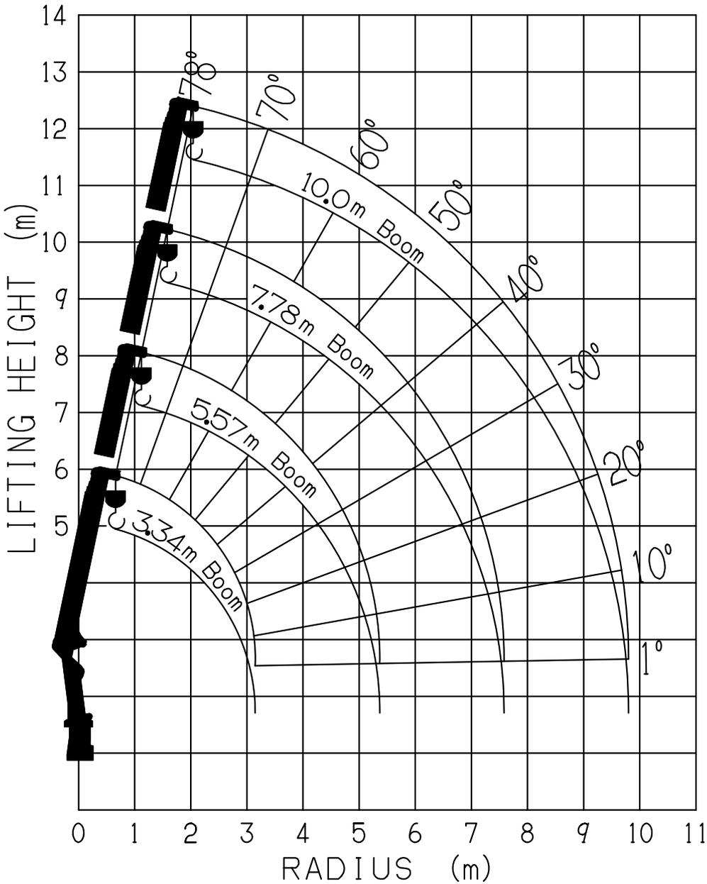
NOTE : The above lifting heights and boom angles are based on a straight (unladen) boom, and allowance should be made for boom deflection obtained under laden conditions.
