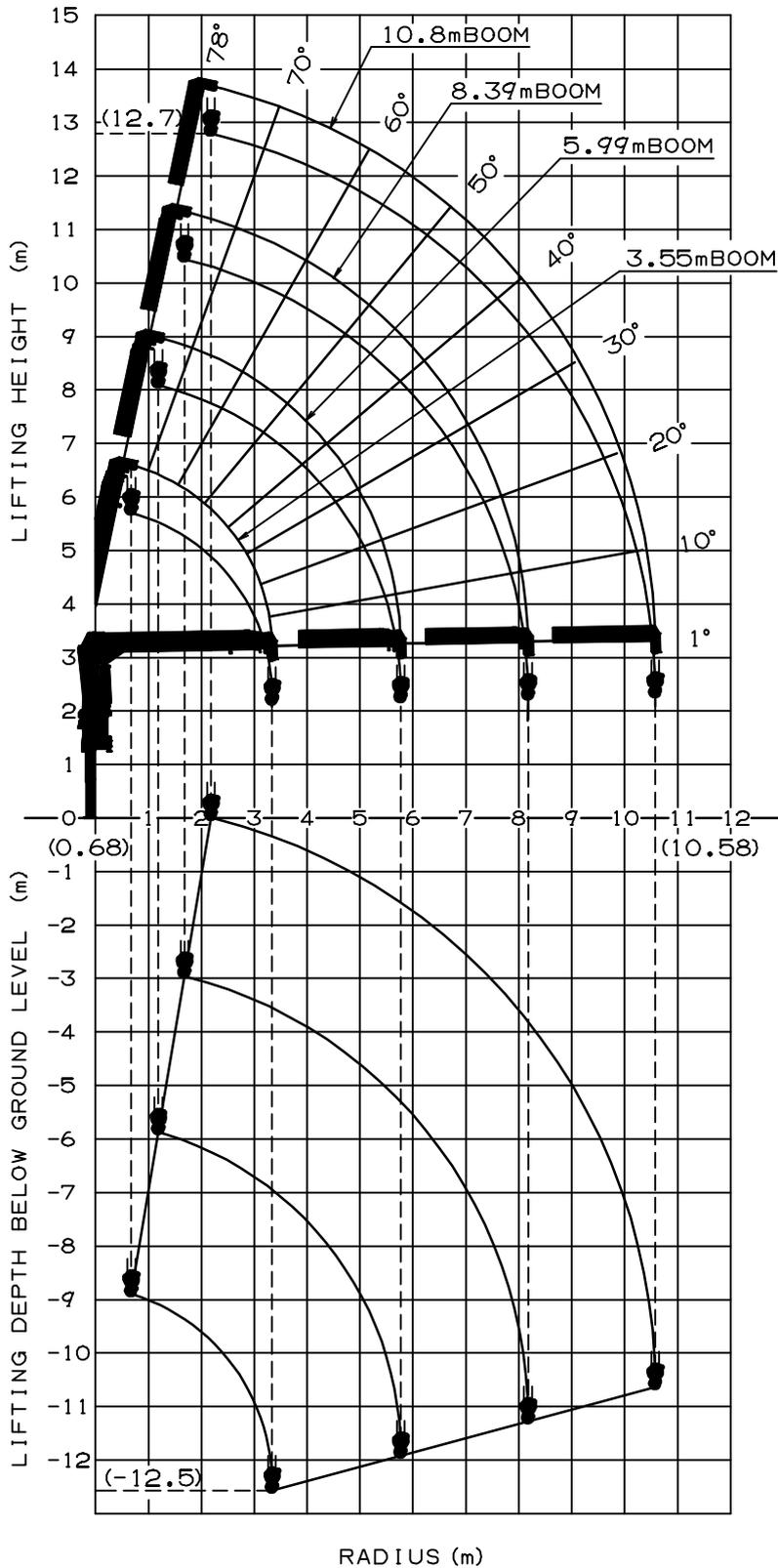
NOTE: The above lifting heights and boom angles are based on a straight (unladen) boom, and allowance should be made for boom deflection obtained under laden conditions.
