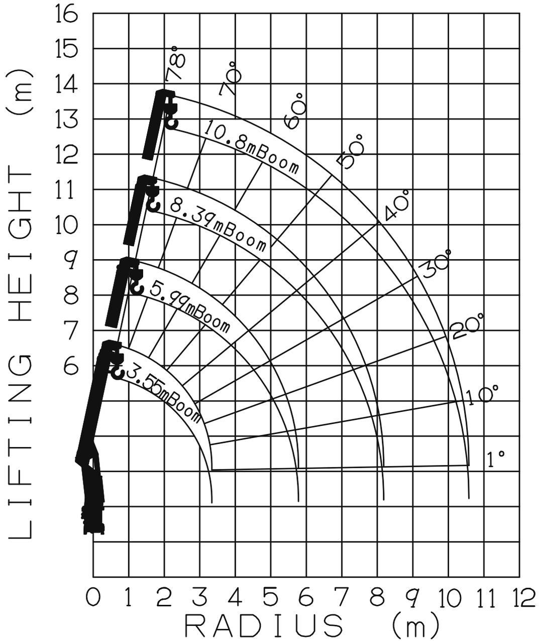
NOTE: The above lifting heights and boom angles are based on a straight (unladen) boom, and allowance should be made for boom deflection obtained under laden conditions.
