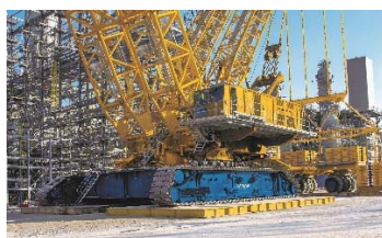
Demag Crawler Crane (CC 8800-1 TWIN)
