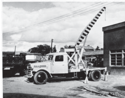
The OC-2 hydraulic truck crane
