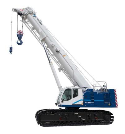
telescopic boom and the integration of Tadano winches, jib, hydraulic cylinders, AML-C and Hello Net telematics.
