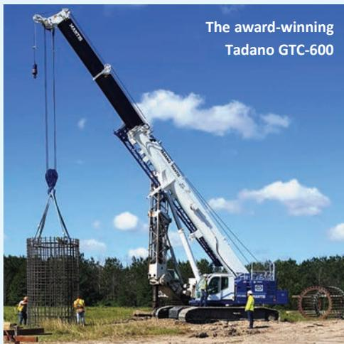
Series. The design project was managed by Tadano Mantis and included collaboration with Tadano Ltd in developing the purpose-designed, Tadano-built telescopic boom and the integration of Tadano winches, jib, hydraulic cylinders, AML-C rated capacity indicator and Hello-Net telematics.
