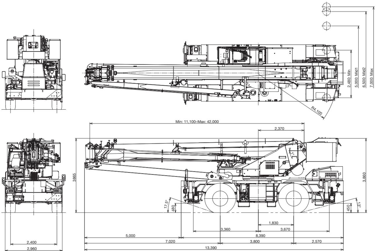
Note : Dimension is with boom angle at -1 degree.
