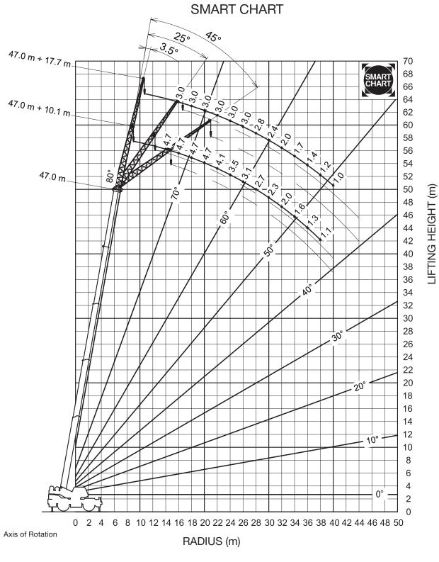
NOTE: 1.Jib geometry shown is for unloaded condition and machine standing level on firm supporting surface. Boom deflection and subsequent radius and boom angle change must be
