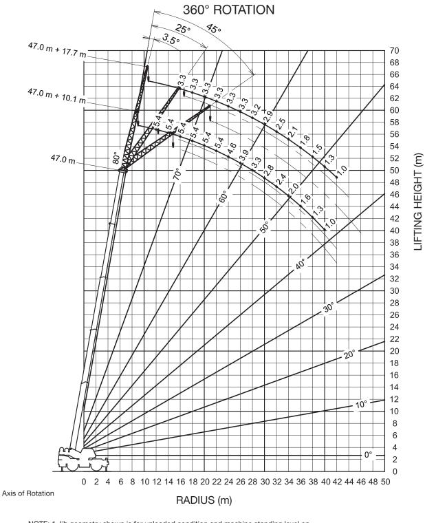
NOTE: 1.Jib geometry shown is for unloaded condition and machine standing level on firm supporting surface. Boom deflection and subsequent radius and boom angle change must be
