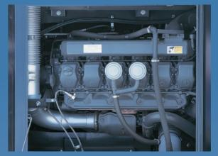
The engine used in this model of crane is made by Daimler and has a maximum output of 260 kW. It satisfies the EURO I standards and is environment-friendly.
