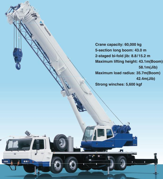
The GT-600EX has a newly developed rounded solid boom of 43.0 m—the longest boom in its class. In addition, with the introduction of a new Automatic Moment Limiter model, the AML-C offers customers a safer operating environment. Further, improved traveling performance ensures a comfortable drive to work sites.
