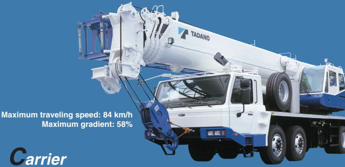
A high-performance engine that meets the EURO III standards is mounted on the carrier. The steering ability of the wheel when the carrier is in a stop condition, along with the adoption of a new hydraulic suspension system, substantially improves the mobility of the crane. In addition, the flat carrier fender eases access to the upper structure.
