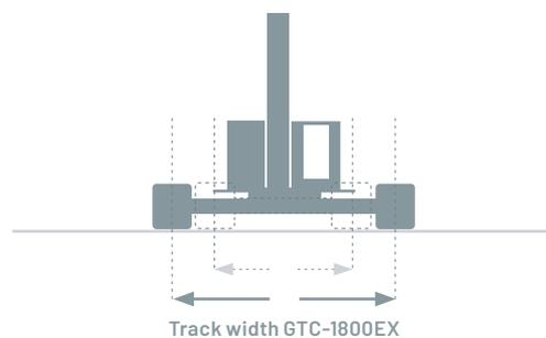
The track width is continuously variable, symmetrical and asymmetrical, within the range of 3.5 to 6 meters
