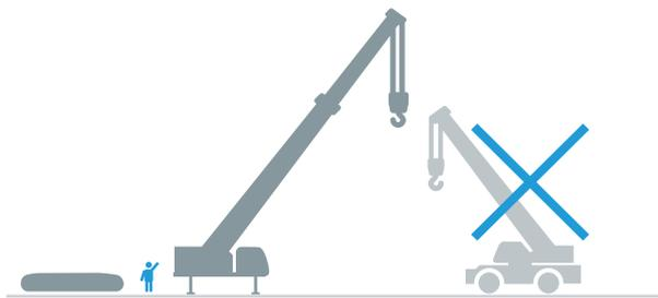
Self-assembly | 1 rigger | no assist crane
