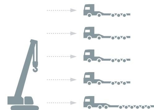
Depending on the application, 1 low-bed truck and 4 standard trucks can carry the base crane and all crane components
