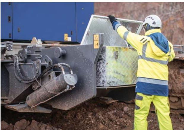
Sufficient space: the lockable aluminum box with a volume of 250 liters is intended for tools and personal items. Chain slings are kept in another large, open box.
