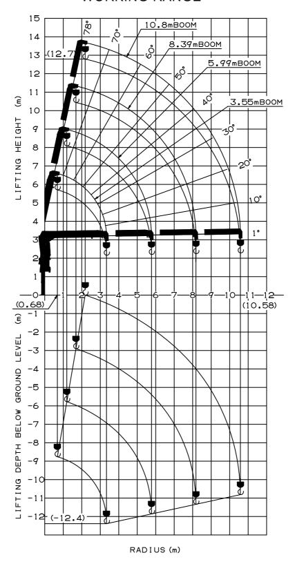
NOTE: The above lifting heights and boom angles are based on a straight (unladen) boom, and allowance should be made for boom deflection obtained under laden conditions.
