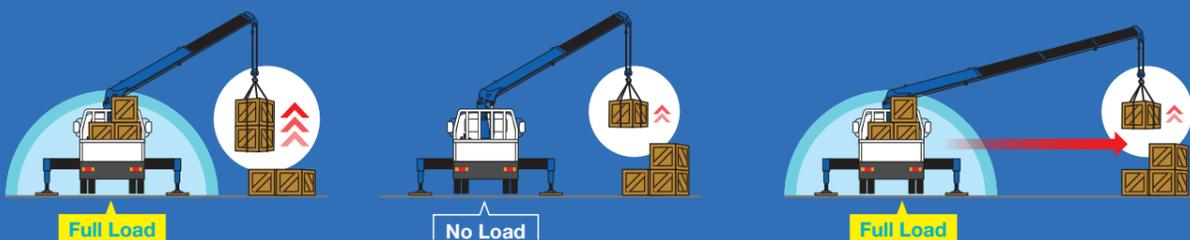
Calculations are automatic based on loaded cargo (stability), allowing you to carry heavier loads farther when fully loaded.
