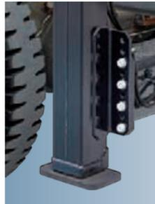
The photo shows outrigger beam non-extension type.
