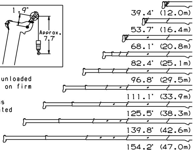
NOTE: 1. Boom and jib geometry shown are for unloaded condition and machine standing level on firm supporting surface. Boom deflection and subsequent radius and boom angle change must be accounted for when applying load to hook.
