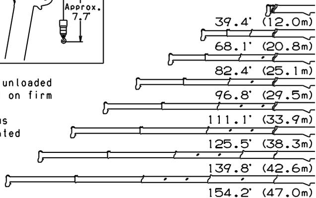
NOTE: 1. Boom and jib geometry shown are for unloaded condition and machine standing level on firm supporting surface. Boom deflection and subsequent radius and boom angle change must be accounted for when applying load to hook.
