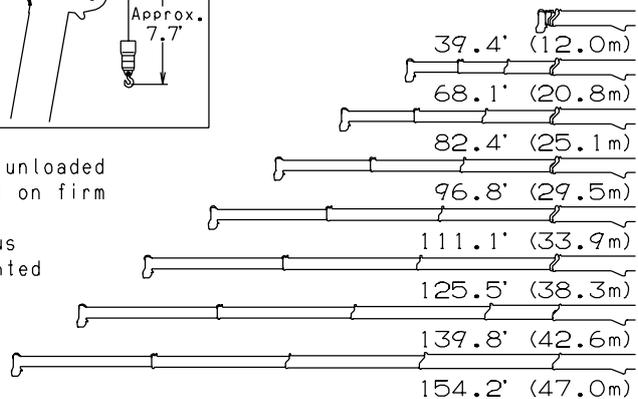
NOTE: 1. Boom and jib geometry shown are for unloaded condition and machine standing level on firm supporting surface.
