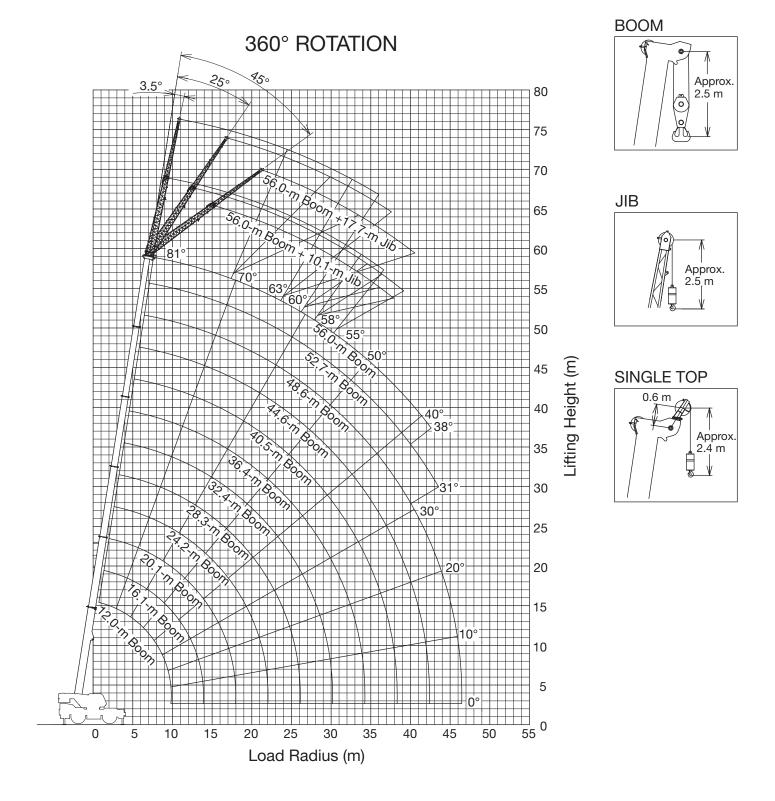
NOTE: Boom and jib geometry shown are for unloaded condition and machine standing level on firm supporting surface.
