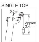
NOTE: Boom geometry shown are for unloaded condition and machine standing level on firm supporting surface. Boom deflection and subsequent radius and boom angle change must be accounted for when applying load to hook.
