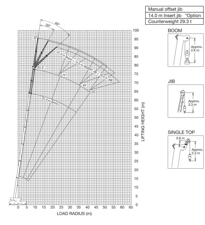
NOTE: Boom and jib geometry shown are for unloaded condition and machine standing level on firm supporting surface. Boom deflection and subsequent radius and boom angle change must be accounted for when applying load to hook.
