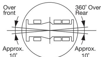
Over front and rear operation shall be performed within 10 degrees.
