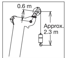
NOTE: Boom and jib geometry shown are for unloaded condition and machine standing level on firm supporting surface. Boom deflection and subsequent radius and boom angle change must be accounted for when applying load to hook.
