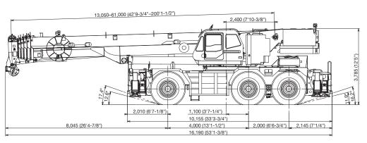
Note: Dimension is with boom angle at -1.5 degree.
