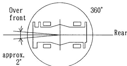
Without outriggers "Over front" operation should be performed within 2 degrees in front of chassis.
