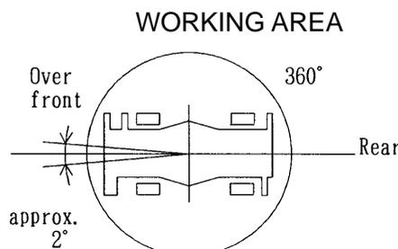
Without outriggers "Over front" operation should be performed within 2 degrees in front of chassis.
