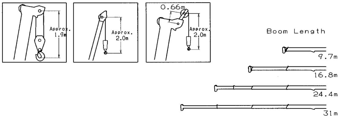
NOTE: The above lifting height and boom angle are based on a straight (unladen) boom, and allowance should be made for boom deflection obtained under laden conditions.
