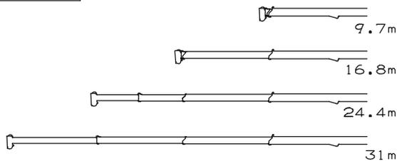
**NOTE:** The above lifting height and boom angle are based on a straight (unladen) boom, and allowance should be made for boom deflection obtained under laden conditions.
