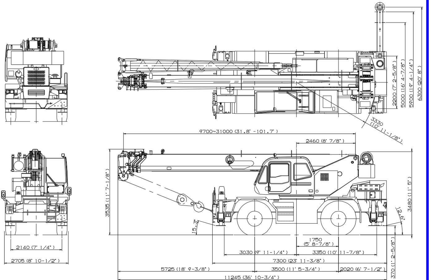
Note : Dimension is with boom angle at 0 degree.
