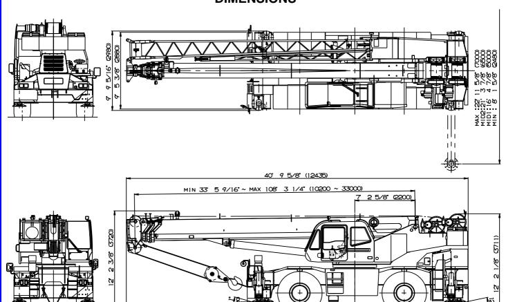
Note: Dimension is with boom angle at -0.8 degree.
