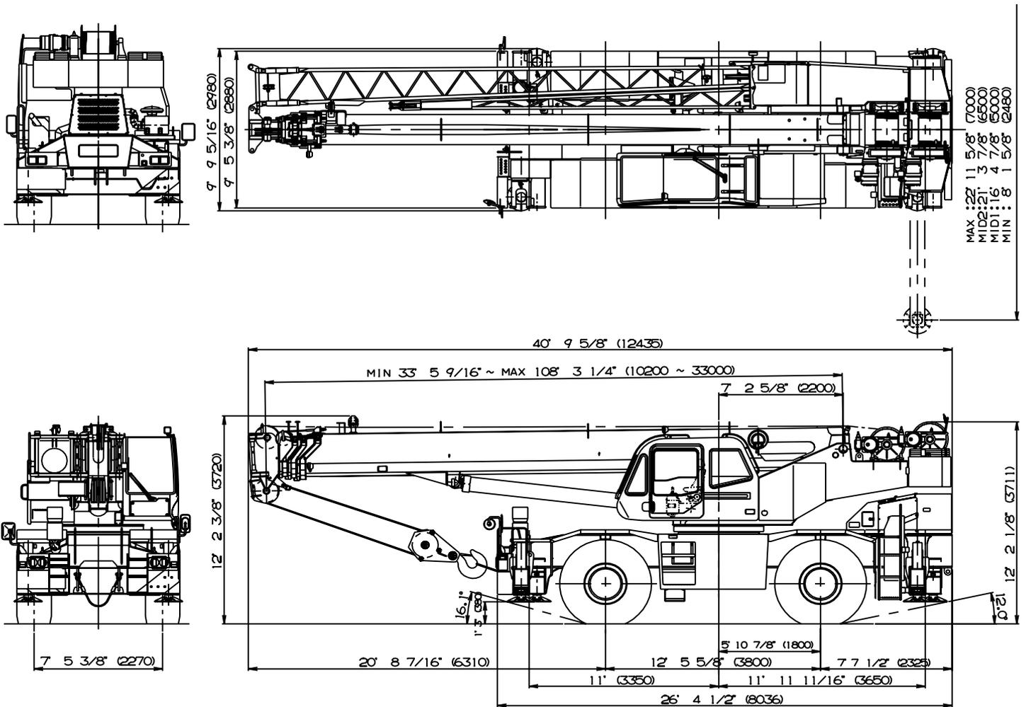
Note : Dimension is with boom angle at -0.8 degree.
