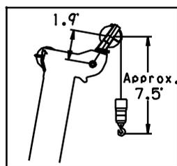
NOTE: Boom and jib geometry shown are for unloaded condition and machine standing level on firm supporting surface. Boom deflection and subsequent radius and boom angle change must be accounted for when applying load to hook.
