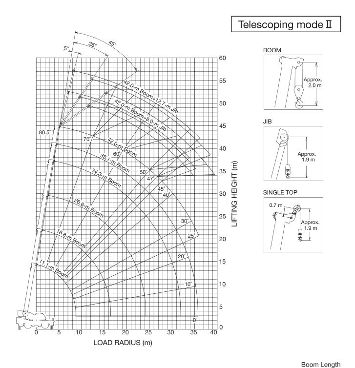
The above lifting height and boom angle are based on a straight (unloaded) boom and machine standing level on firm supporting surface. Allowance should be made for boom deflection obtained under loaded conditions. The above working range is shown on condition with outriggers fully (7.0 m) extended.
