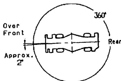
Without outriggers "Over front" operation should be performed within 2 degrees in front of chassis.
