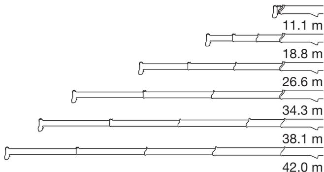
The above lifting height and boom angle are based on a straight (unloaded) boom and machine standing level on firm supporting surface. Allowance should be made for boom deflection obtained under loaded conditions. The above working range is shown on condition with outriggers fully (7.0 m) extended.
