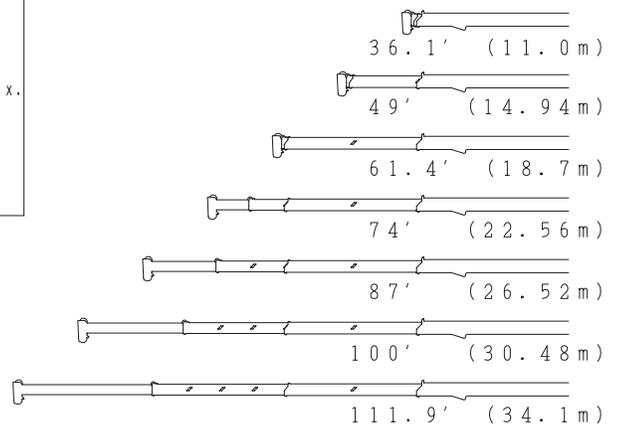
**NOTE :** 1. Boom and jib geometry shown are for unloaded condition and machine standing level on firm supporting surface. Boom deflection and subsequent radius and boom angle change must be accounted for when applying load to hook.
