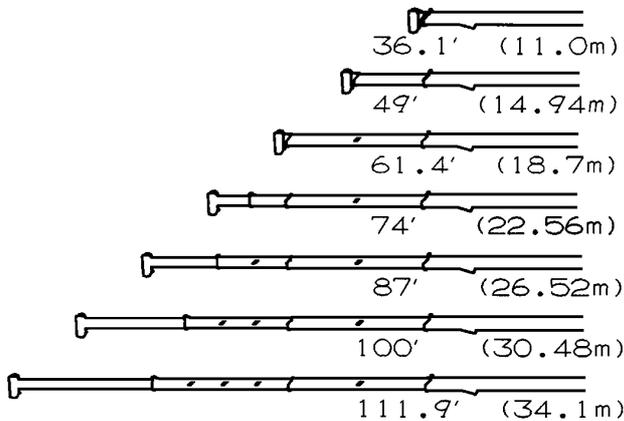
NOTE: Load radiuses for jib operation are given for reference with the boom fully extended to 111.9' (34.1m).
