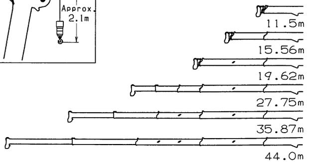
NOTE: The above lifting height and boom angle are based on a straight (unladen) boom, and allowance should be made for boom deflection obtained under laden conditions.
