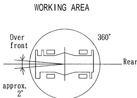
Without outriggers "Over front" operation should be performed within 2 degrees in front of chassis.
