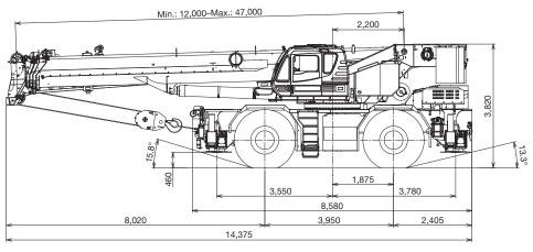
Note: Dimension is with boom angle at -1.6 degree.
