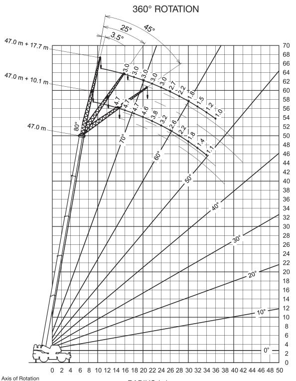
NOTE: 1.Jib geometry shown is for unloaded condition and machine standing level on firm supporting surface.
