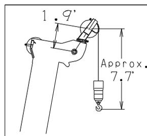
NOTE: 1. Boom geometry shown is for unloaded condition and machine standing level on firm supporting surface. Boom deflection and subsequent radius and boom angle change must be accounted for when applying load to hook.
