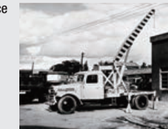
The first hydraulic truck crane, the OC-2
