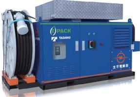
E-Pack: An external power source operates a hydraulic pump driven by an electric motor, enabling crane operation without starting the engine and achieving zero CO2 emissions during operation.
