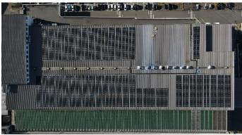
The newly completed solar power generating system has a total panel capacity of 606.8 kW, of which 543,000 kWh is expected to be consumed annually at the company's plant. As a result, it is estimated that 32.2% of annual power consumption at the Tadotsu Plant will be provided by renewable energy.
