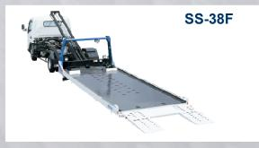
(Slide bed Vehicle Carrier [transport vehicle])
