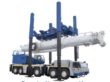
Example of boom removal from All Terrain Crane, ATF400G CL-500 (Released on August 2013)
