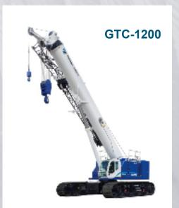
(Introduced March 2015 First TMC model to use a round boom, developed jointly with TADANO)
