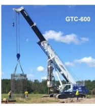
Launched in January 2017 Features highly lauded 'Opti-Width' function and capability of working out of level.
