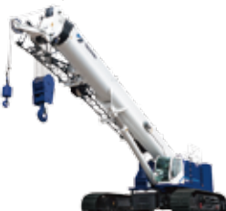
(6) Telescopic boom crawler crane
